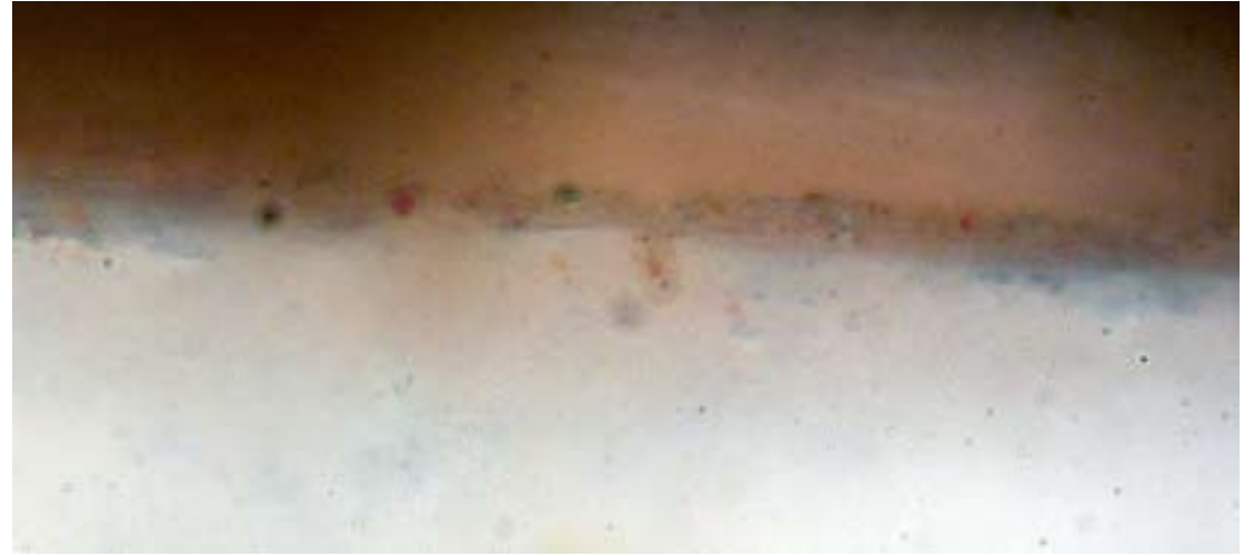
Cross-section of sample 3804 (photographed at 100x) showing the upper plaster layer taken from the west wall of the exterior of the Sheesh Mahal. The cross-section shows a translucent coating on the surface of the plaster.
