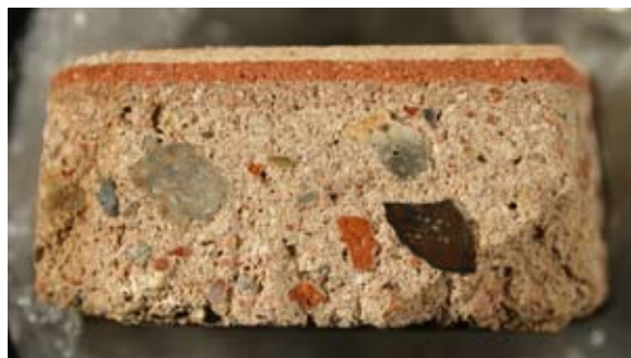
Left: a plaster sample (width 3 cm) from the Sheesh Mahal showing a coarse lime plaster layer with large aggregates and brick particles, finer layer composed of brick powder and lime, and the uppermost fine polished lime and marble powder layer.
