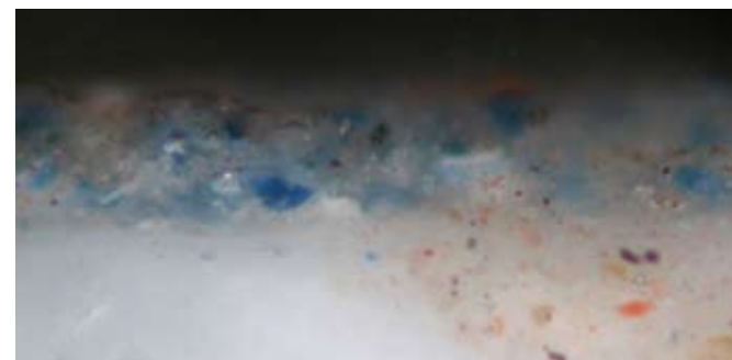
Above and left: the exterior scheme of Sheesh Mahal retains an unaltered blue pigment which is probably smalt (Sample #3793, 200x).
