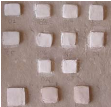
Plaster tests used in the development and selection of a suitable repair material.
